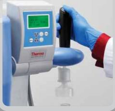
Exact dosing from GenPure Pro water purification system with one touch dispensing
