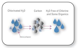
feed water with organic and chlorine contaminants come into contact with the activated carbon in the cartridge.
