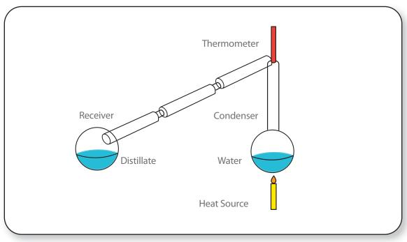
A basic distillation diagram.
