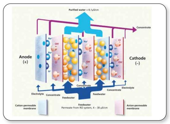
Process of electrodeionization
