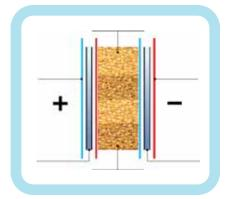
Electrodeionization, EDI, unites two proven technologies for producing ultrapure water: Electrodialysis and ion exchange. In contrast to conventional ion exchange in which resins must be either chemically regenerated or the cartridge discarded, EDI utilizes an electric current for continual resin regeneration.
