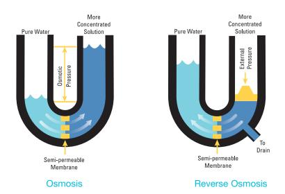
The natural osmosic flow of water through a semi-permeable membrane from less concentrated solutions to more concentrated solutions. Reverse osmosis is achieved when external pressure is applied to reverse this natural flow, as shown on the right.
